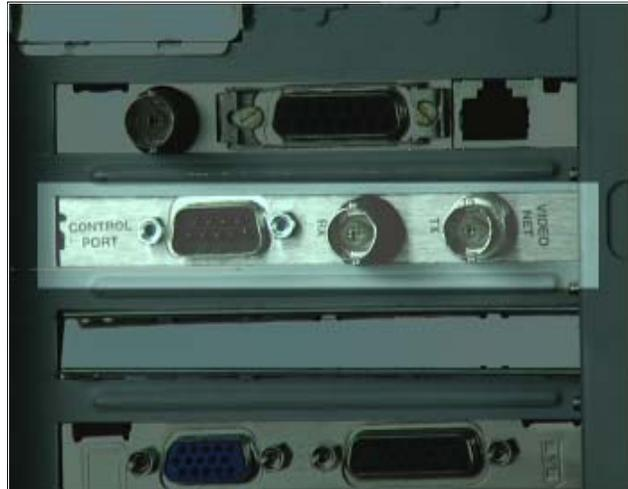
*Figure 3.3: The TX And RX Connectors On The VideoNet Card*
