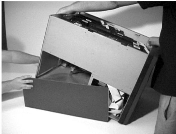
*Figure 4.11: Removing the Bottom Cover of GlobeCaster*
