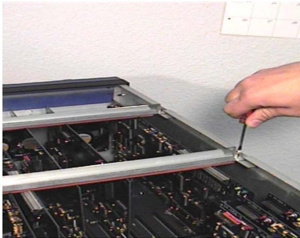
*Figure 3.17: Removal of Retaining Bar*
