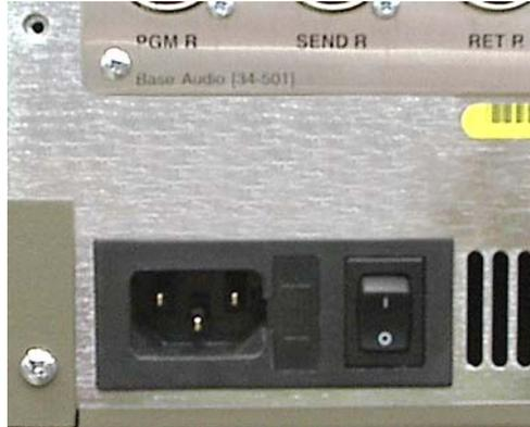
Figure 3.6: The Power Connector On The GlobeCaster Hardware
