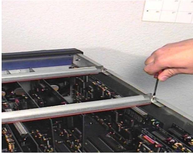
Figure 4.12: Removal of Retaining Bar
