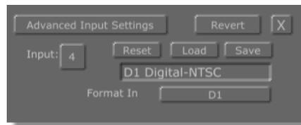
Figure 6.10: Advanced Input Settings Panel for Serial Digital Input Card
