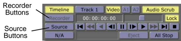
Figure 5.9: The Source and Recorder Buttons
