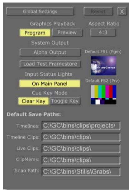
Figure 5.2: Turning on the Input Status Lights
