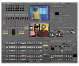
Graphics over video (upper left), picture-inpicture (middle left), dissolve between keyed and non-keyed sources (bottom left) and preview keyed sources and virtual set panel directly from the Switcher interface (above).
